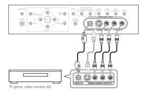
Select these inputs using INPUT SELECT (remote) or the INPUT SELECTOR dial (front panel) to select VIDEO/GAME 2.
